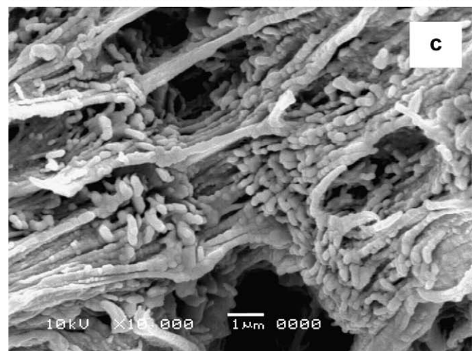
Fig. 15. SEM micrographs of surface of fractured tensile specimen of PLA/PPG4-7.5 (a), PLA/PPG4-12.5: overview (b) and detail (c).
